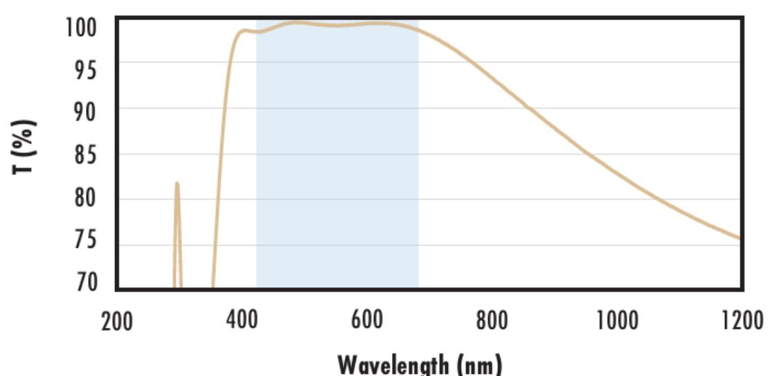
Typical transmission of a 3mm thick fused silica window with VIS 0° (425-675nm) coating at 0° AOI.
