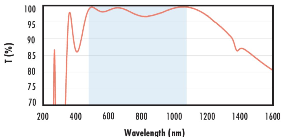
Typical transmission of a 3mm thick fused silica window with YAG-BBAR (500-1100nm) coating at 0° AOI.
