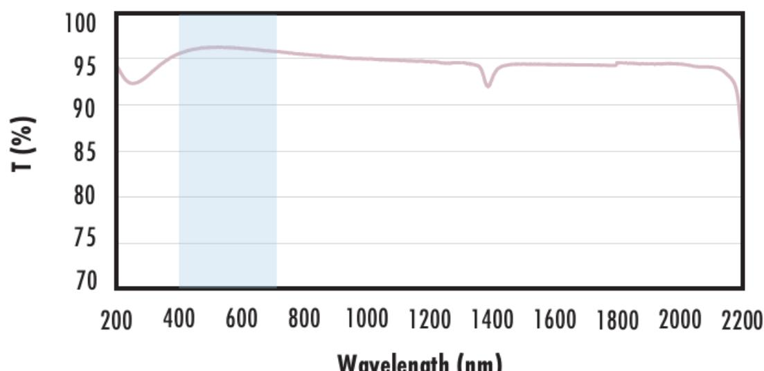
Typical transmission of a 3mm thick fused silica window with  $MgF_2$  (400-700nm) coating at 0° AOI.
