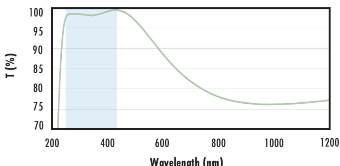
Typical transmission of a 3mm thick fused silica window with UV-AR (250-425nm) coating at 0° AOI.
