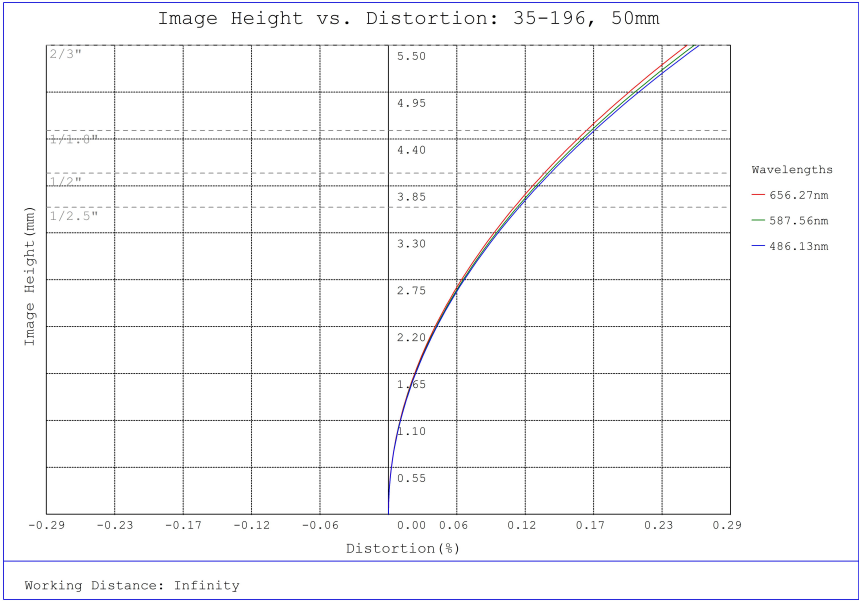
#35-196, 50mm, f/16 Cr Series Fixed Focal Length Lens, Distortion Plot
