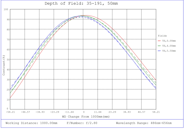
#35-191, 50mm, f/2.8 Cr Series Fixed Focal Length Lens, Depth of Field Plot, 1000mm Working Distance, f2.8
