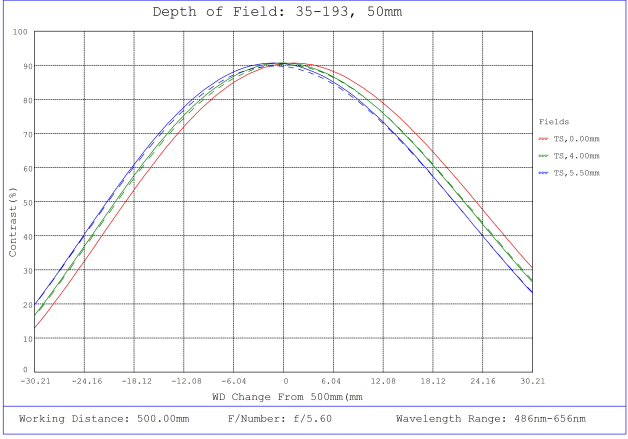
#35-193, 50mm, f/5.6 Cr Series Fixed Focal Length Lens, Depth of Field Plot, 500mm Working Distance, f5.6
