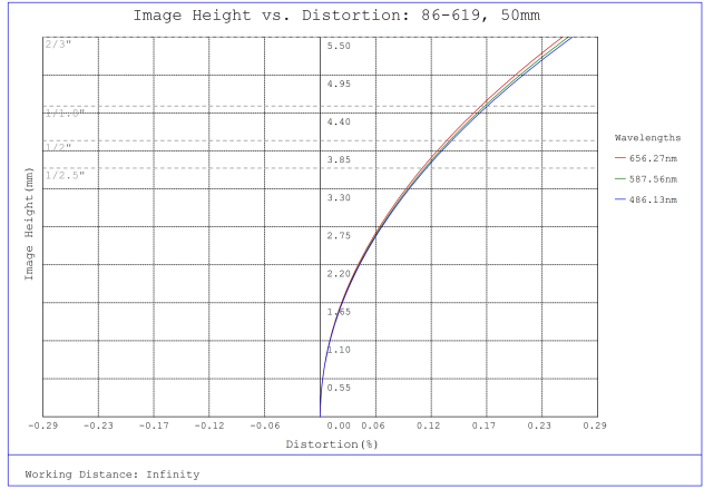
#86-619, 50mm, f/11.0 Ci Series Fixed Focal Length Lens, Distortion Plot
