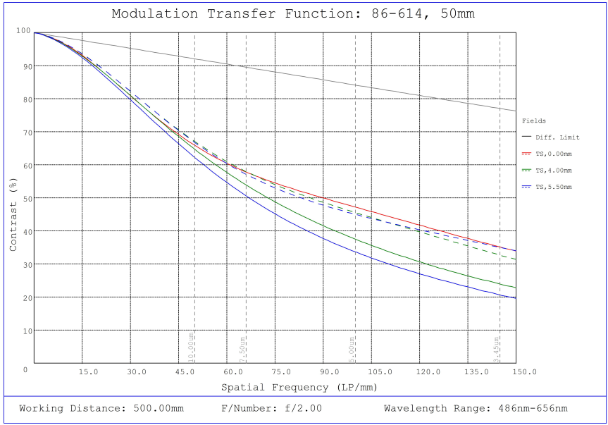
#86-614, 50mm, f/2.0 Ci Series Fixed Focal Length Lens, Modulated Transfer Function (MTF) Plot, 500mm Working Distance, f2
