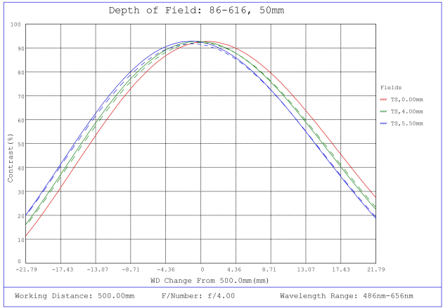
#86-616, 50mm, f/4.0 Ci Series Fixed Focal Length Lens, Depth of Field Plot, 500mm Working Distance, f4
