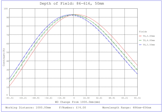
#86-616, 50mm, f/4.0 Ci Series Fixed Focal Length Lens, Depth of Field Plot, 1000mm Working Distance, f4
