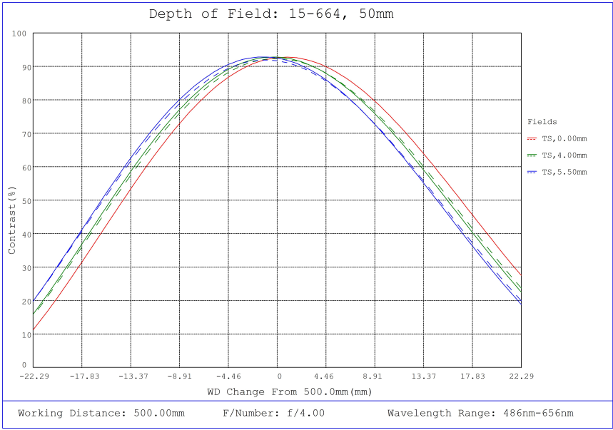
#15-664, 50mm, f/4.0 Sealed Cw Series Fixed Focal Length Lens, Depth of Field Plot, 500mm Working Distance, f4
