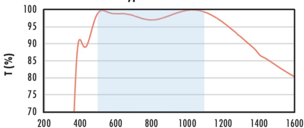
Typical transmission of a 3mm thick N-BK7 window with YAG-BBAR (500-1100nm) coating at 0° AOI.
