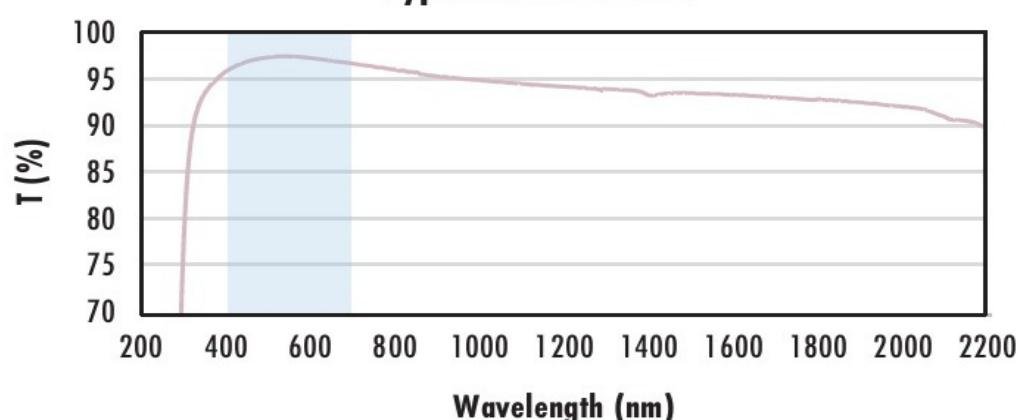
Typical transmission of a 3mm thick N-BK7 window with MgF<sub>2</sub> (400-700nm) coating at 0° AOI.
