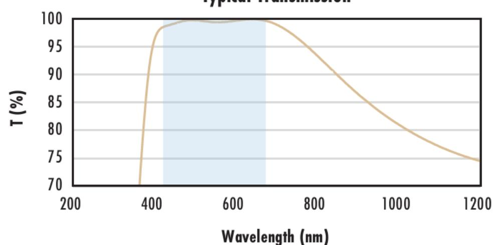
Typical transmission of a 3mm thick N-BK7 window with VIS 0° (425-675nm) coating at 0° AOI.
