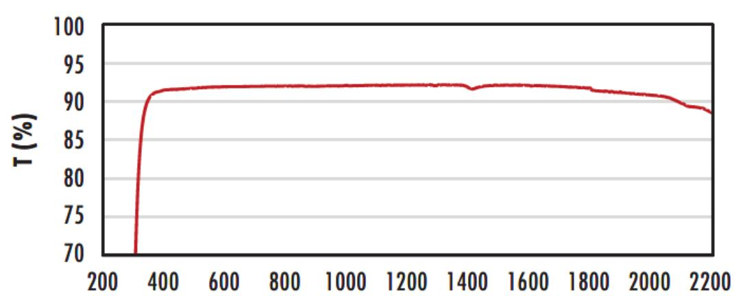
Typical transmission of a 3mm thick, uncoated N-BK7 window across the UV- NIR spectra.
