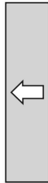
All mounted TECHSPEC® Optical Filters have an arrow on the side of the mount that points to the filter-coated surface for quick reference. Filter oriented such that arrow points to filter coated surface S1. Anti-reflective (AR) coating is applied to S2.
