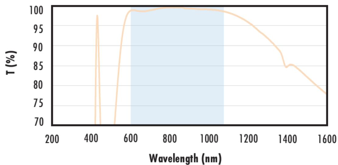
Typical transmission of a 3mm thick fused silica window with NIR I (600 - 1050nm) coating at 0° AOI.
