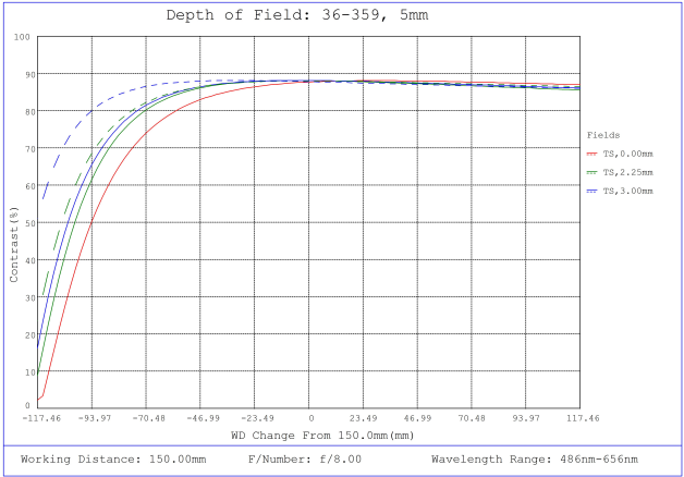
#36-359, 5mm FL f/8, Rugged Blue Series M12 Lens, Depth of Field Plot, 150mm Working Distance, f8
