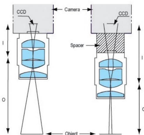
Using C-Mount Spacers in Electronic Imaging
