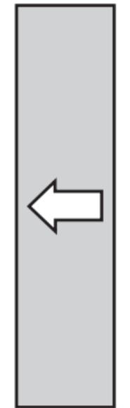
All mounted TECHSPEC® Optical Filters have an arrow on the side of the mount that points to the filter-coated surface for quick reference. Filter oriented such that arrow points to filter coated surface S1.
