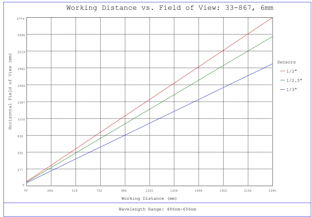
#33-867, 6mm, f/11 UCi Series Fixed Focal Length Lens, Working Distance versus Field of View Plot
