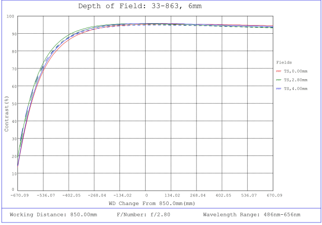
#33-863, 6mm, f/2.8 UCi Series Fixed Focal Length Lens, Depth of Field Plot, 850mm Working Distance, f2.8
