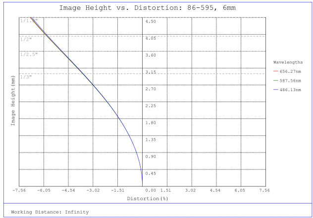
#86-595, 6mm, f/5.6 Ci Series Fixed Focal Length Lens, Distortion Plot
