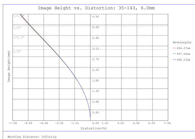
#35-143, 6mm, f/5.6 Cr Series Fixed Focal Length Lens, Distortion Plot
