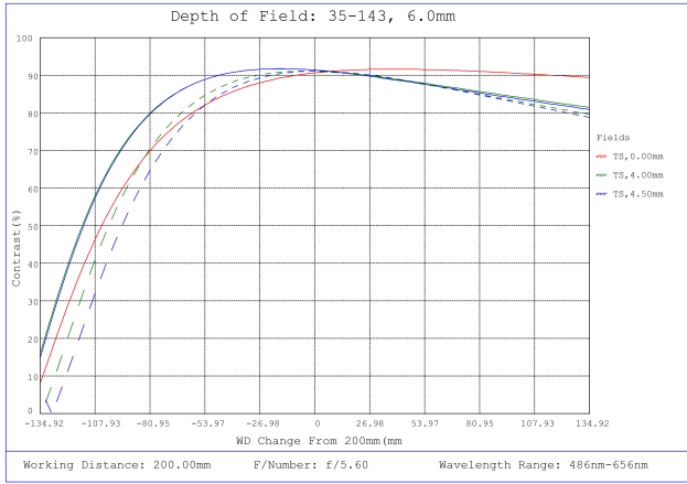
#35-143, 6mm, f/5.6 Cr Series Fixed Focal Length Lens, Depth of Field Plot, 200mm Working Distance, f5.6
