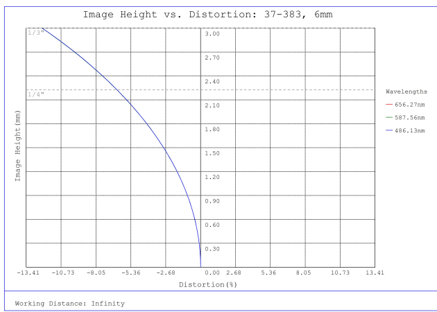
#37-383, 6mm FL f/4.0 , Rugged Blue Series M12 Lens, Distortion Plot
