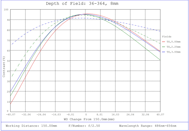
#36-364, 8.0mm FL f/2.5, Rugged Blue Series M12 Lens, Depth of Field Plot, 150mm Working Distance, f2.5
