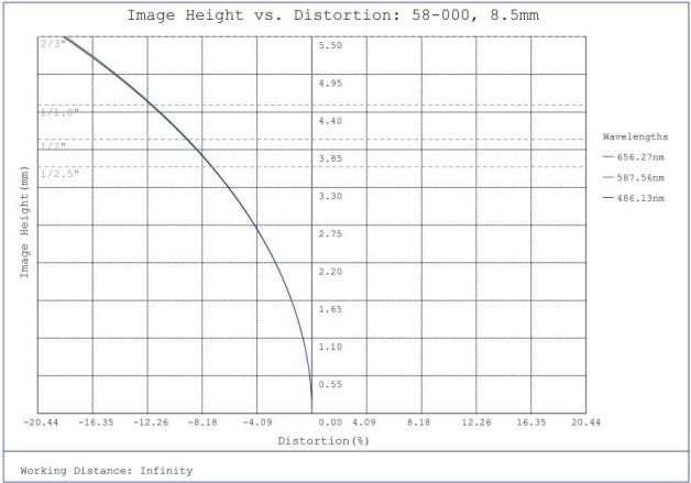
#58-000, 8.5mm C Series Fixed Focal Length Lens, Distortion Plot
