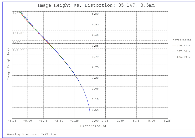
#35-147, 8.5mm, f/1.8, 75mm-∞ Primary WD, HRr Series Fixed Focal Length Lens, Distortion Plot
