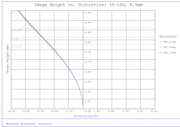
#35-150, 8.5mm, f/4.0, 75mm-∞ Primary WD, HRr Series Fixed Focal Length Lens, Distortion Plot
