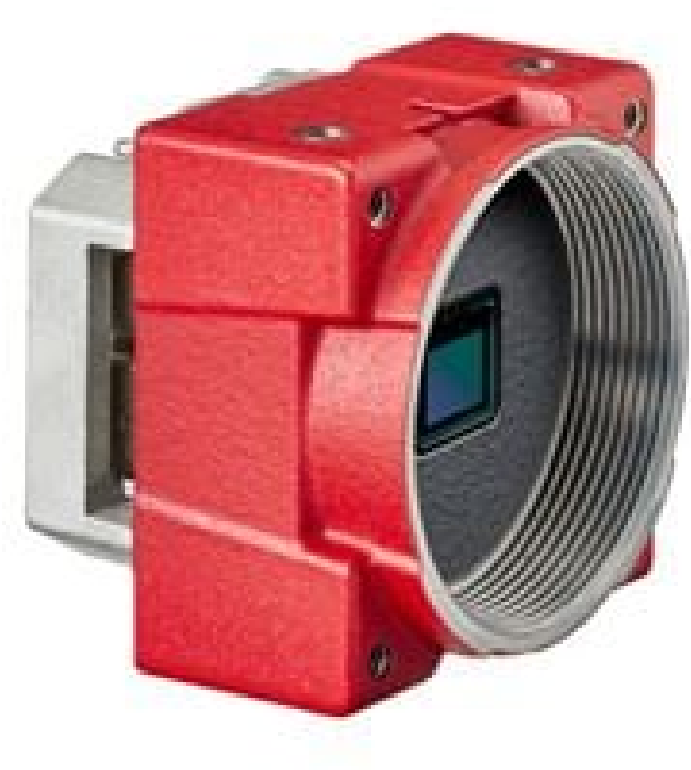
Allied Vision Alvium Camera, Partial Housing, CS-Mount (Front)
