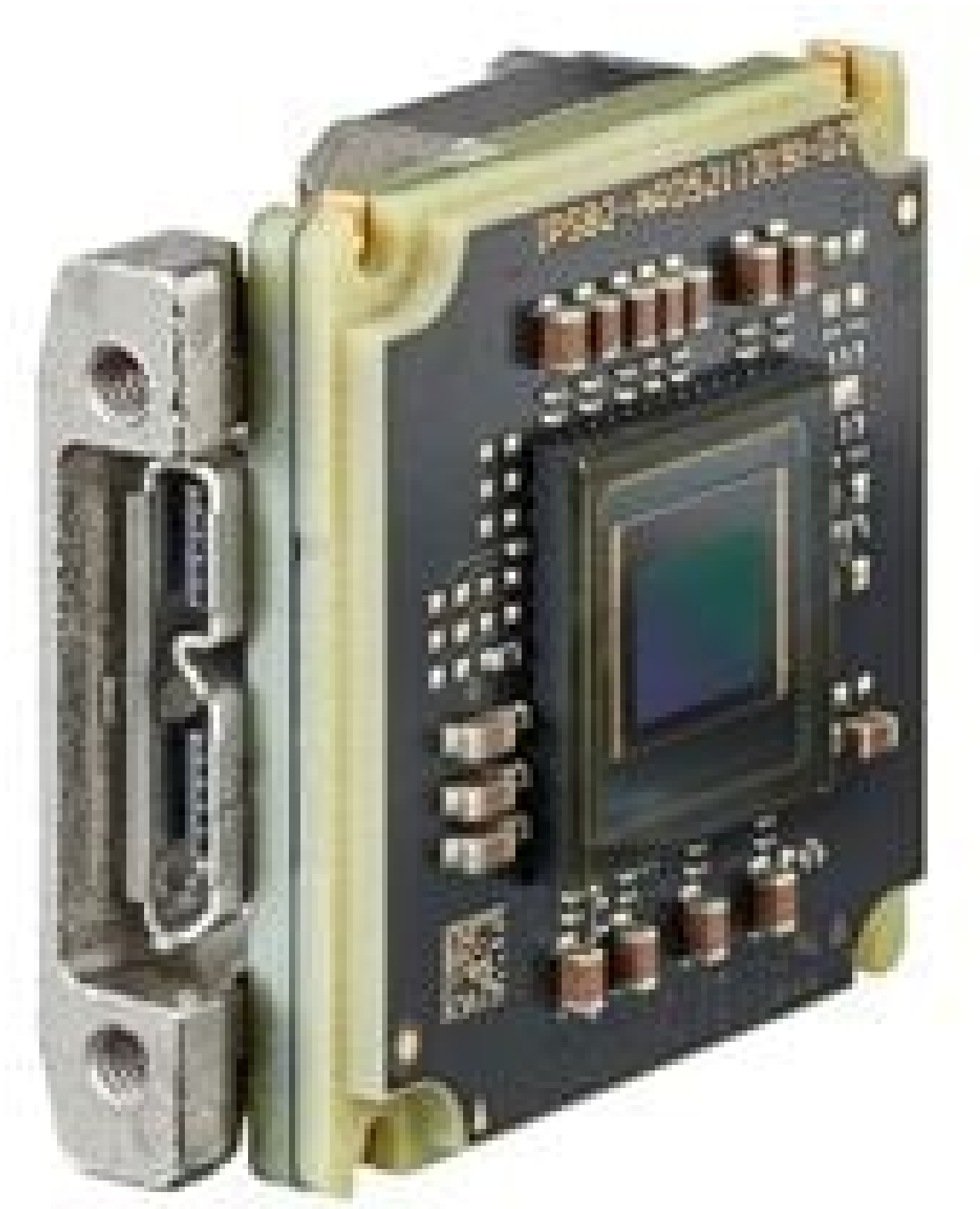
Allied Vision Alvium Camera, Board Level, Right Angle IO Port (Front)
