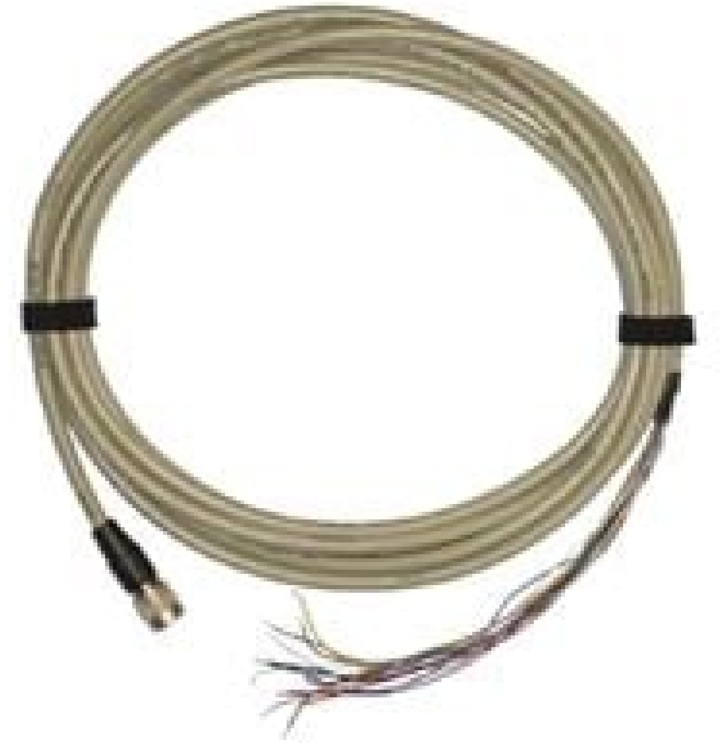
#59-736 Mako GigE, Guppy 5m I/O Breakout Cable
