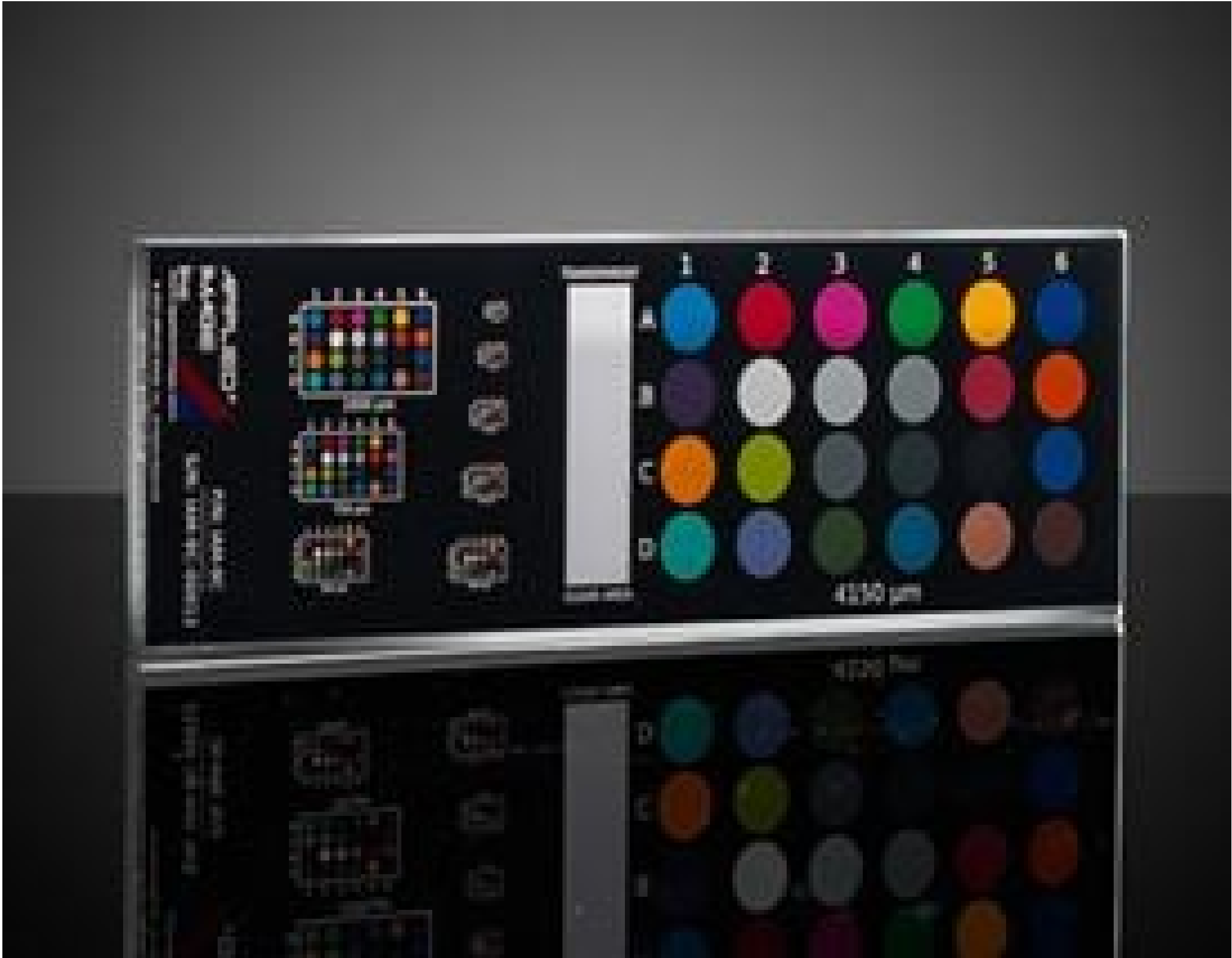
NIST Traceable Color Transmission Calibration Slides
